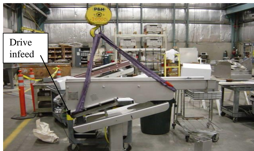
Fig. 3b: VF CONVEYOR ATTACHED TO HOIST
