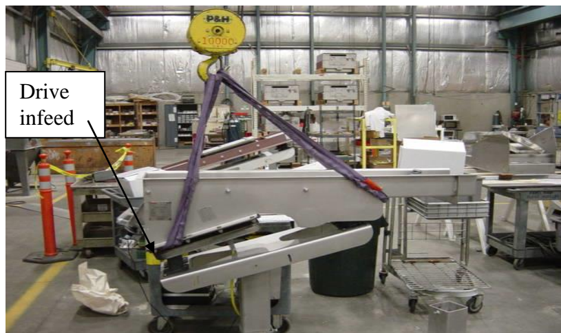
Fig. 3b: VF CONVEYOR ATTACHED TO HOIST
